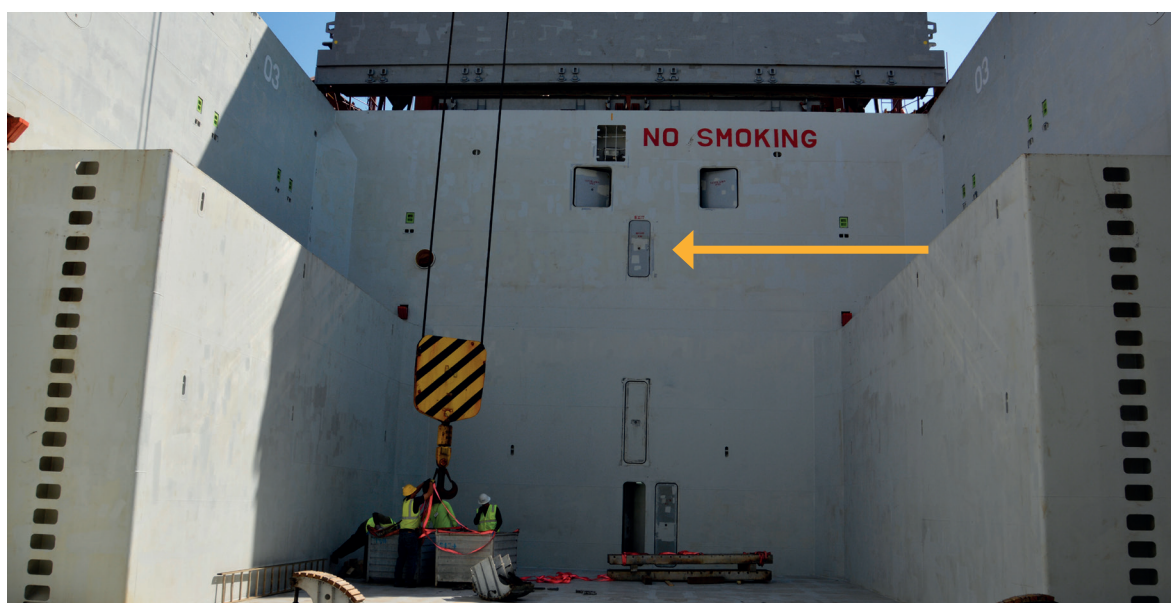
Figure 7: Comparable situation of the doors on the other side of the hold. The deckhand fell into the hold from a door opening at the height marked with the arrow.
