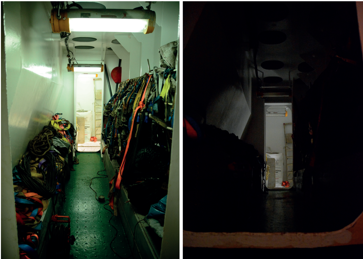
Figure 6: Stairwell where the welding cables were located, with the lighting on/off. These photographs were taken during the visit to the Fortunagracht, two weeks following the accident. On that occasion, the conditions were different from the conditions on the day of the accident. These photographs therefore provide only an indication of the difference between the situation with the lighting switched on and off.
