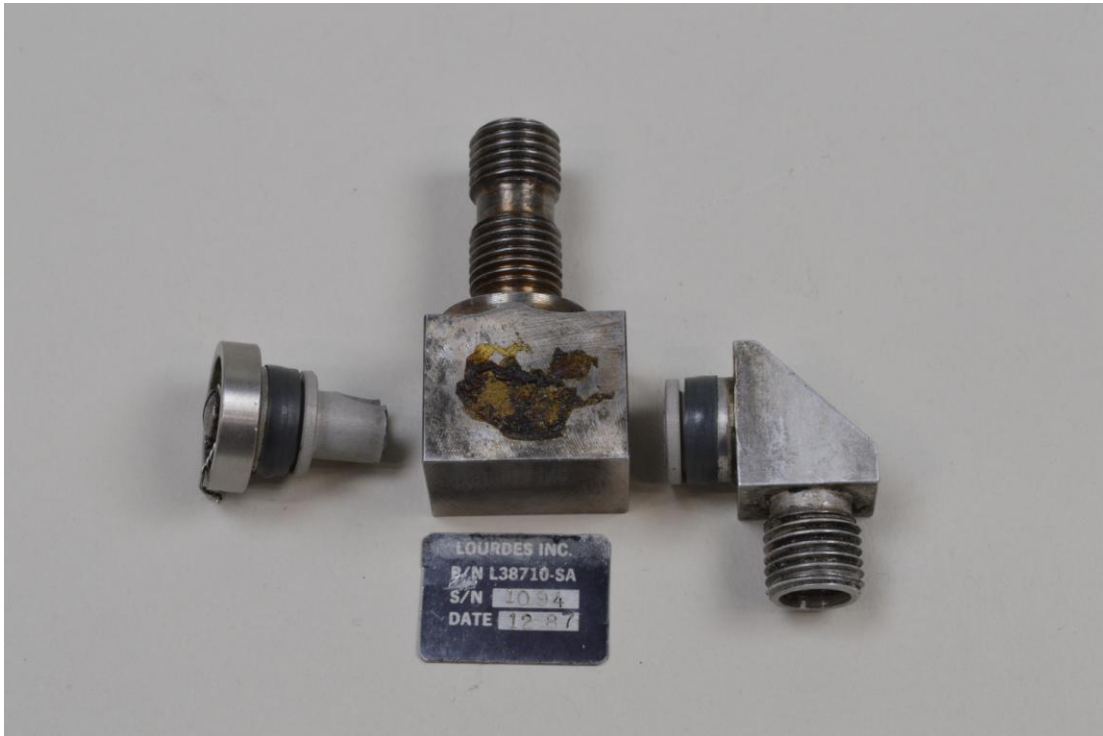
Figure 1. The broken swivel in the as received condition.
