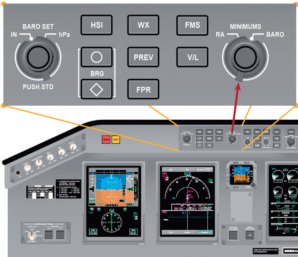
Figure 1: Location of the BARO/RA selection knob on the instrument panel (see red arrow). (Photo: Embraer)
