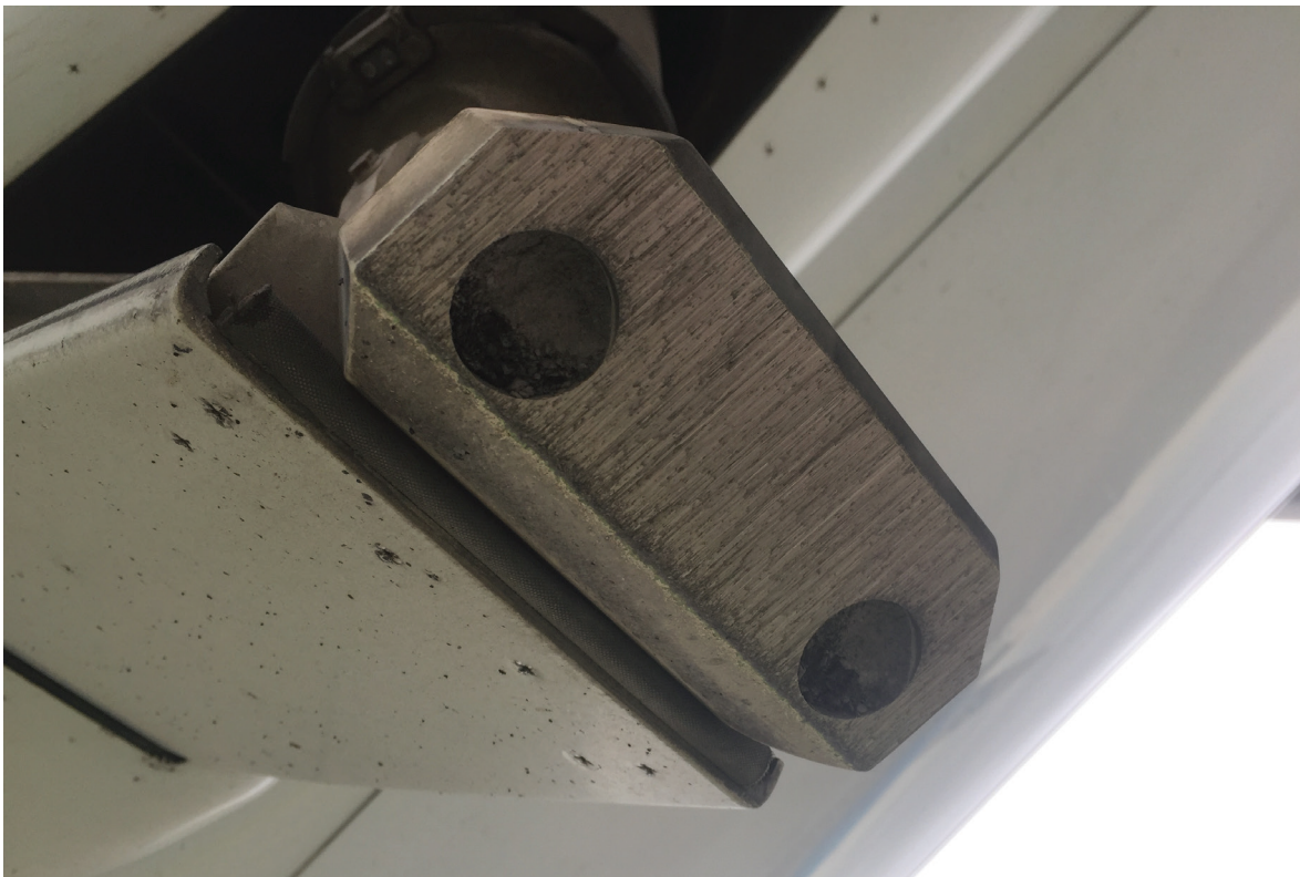
Figure 3: Tail skid shoe with scrape marks.
