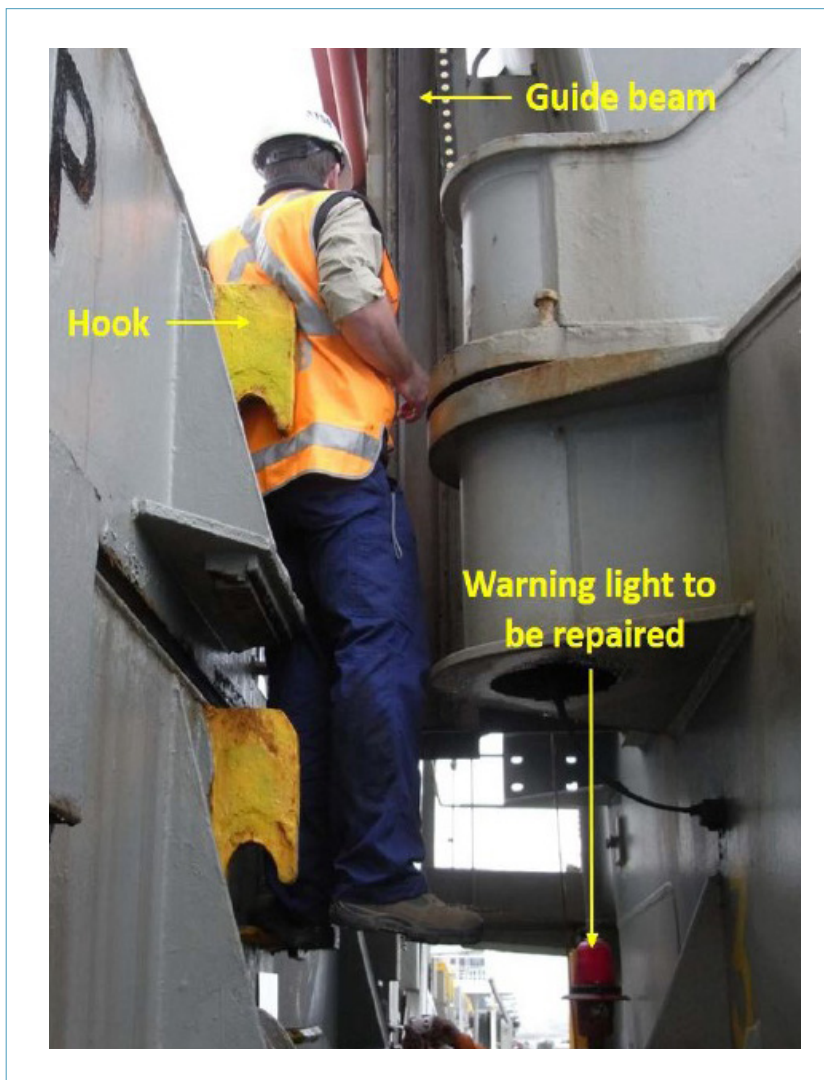
Figure 12: Reconstruction of the occurrence; the victim was probably standing on a ladder of the stacked hatches. (Source: ATSB)
