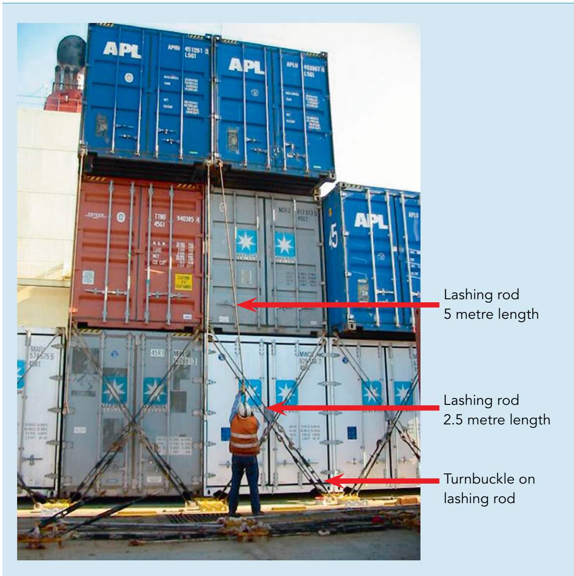
Figure 1: Stevedore secures a 5-metre-long lashing rod. (Source: www.portpictures.nl - Danny Cornelissen)
