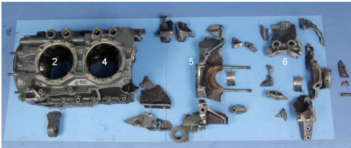
Figure 3: Overview of the crankcase components. The numbers indicate the cylinder positions. (Source: NTSB)
