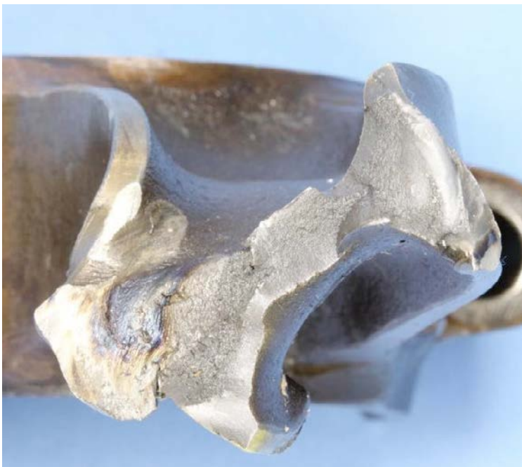
Figure 5: Fractured surface of the number 5 connecting rod. (Source: NTSB)
