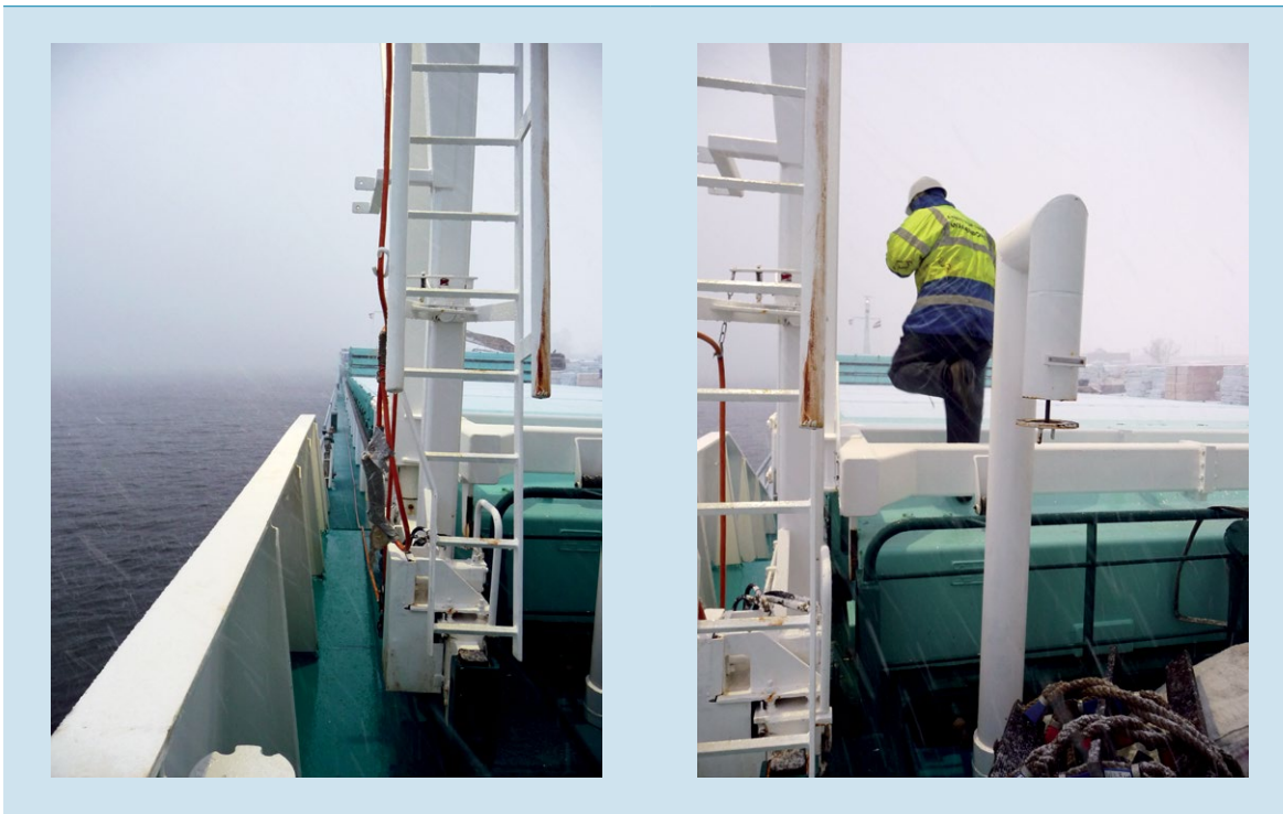
Figure 5: The two options for a passage to the foredeck. Via the gangway (L) or over the deck hatches (R). (Source: Dutch Safety Board)
