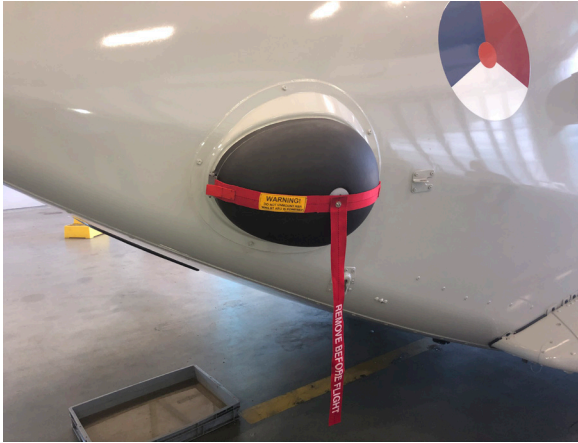
Figure 3, left: Position of the RBA on the outside of the reference aircraft. (Source: Dutch Safety Board) Figure 4, right: The RBA upon transfer at the Parera Naval Base. (Source: Dutch Safety Board)
