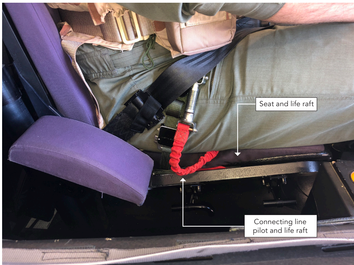
Figure 7: Example of the seating position of the pilot on the seat and life raft with connecting line. (Source: Dutch Safety Board)
