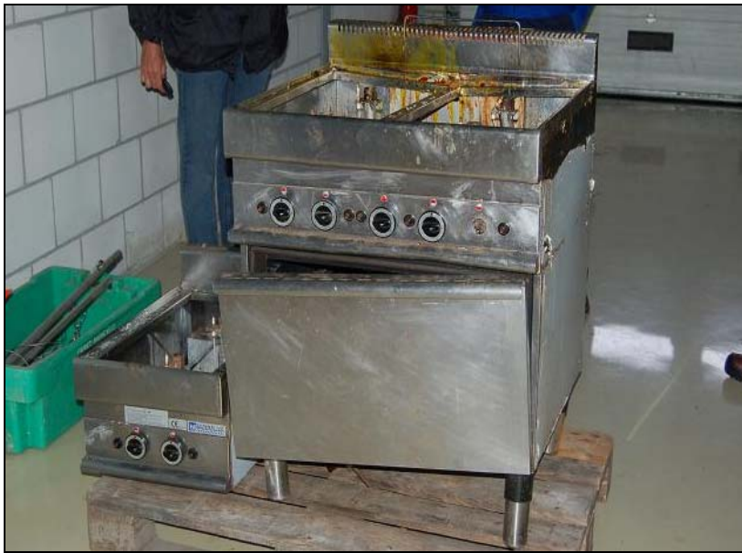
Figure 12: Cooker ready to be taken away for further investigation, with those control knobs present having been turned to the off position (Note: The oven knob is the 3 rd from left - a gas burner knob on the right is missing) (photo: TNO Construction and Service)
