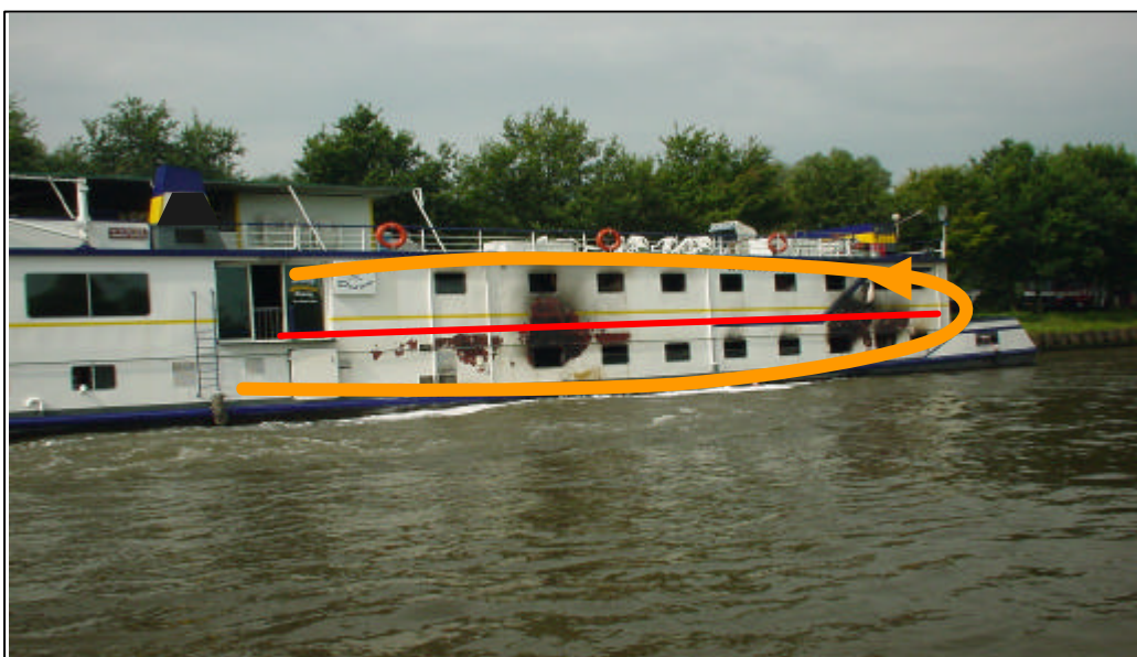
Figure 4: The steel deck is shown in red, the path of the fire in orange: the fire started in the engine room, spreading across the lower deck where the cabins for both the crew and passengers are situated, to the middle deck, where further passenger cabins are situated (Source: Dutch Safety Board).
