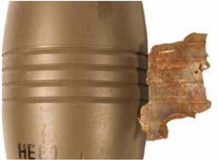
Figure 11: Imprint on the fragment of the launch tube, originating from the grooves on the shell casing when the main charge explodes. Figure illustrates the steel fragments produced during detonation of an HE 80 mortar round. (Picture: TNO)
