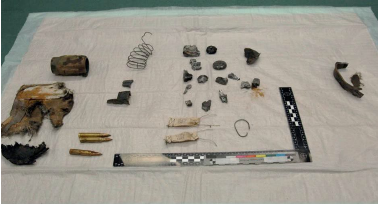
Figure 7: Content of the paper bag: visible are the same parts as in Figure 6, parts of a magazine and (probably) a part of the carrier/firing belt of the mortar. (Picture: TNO)
