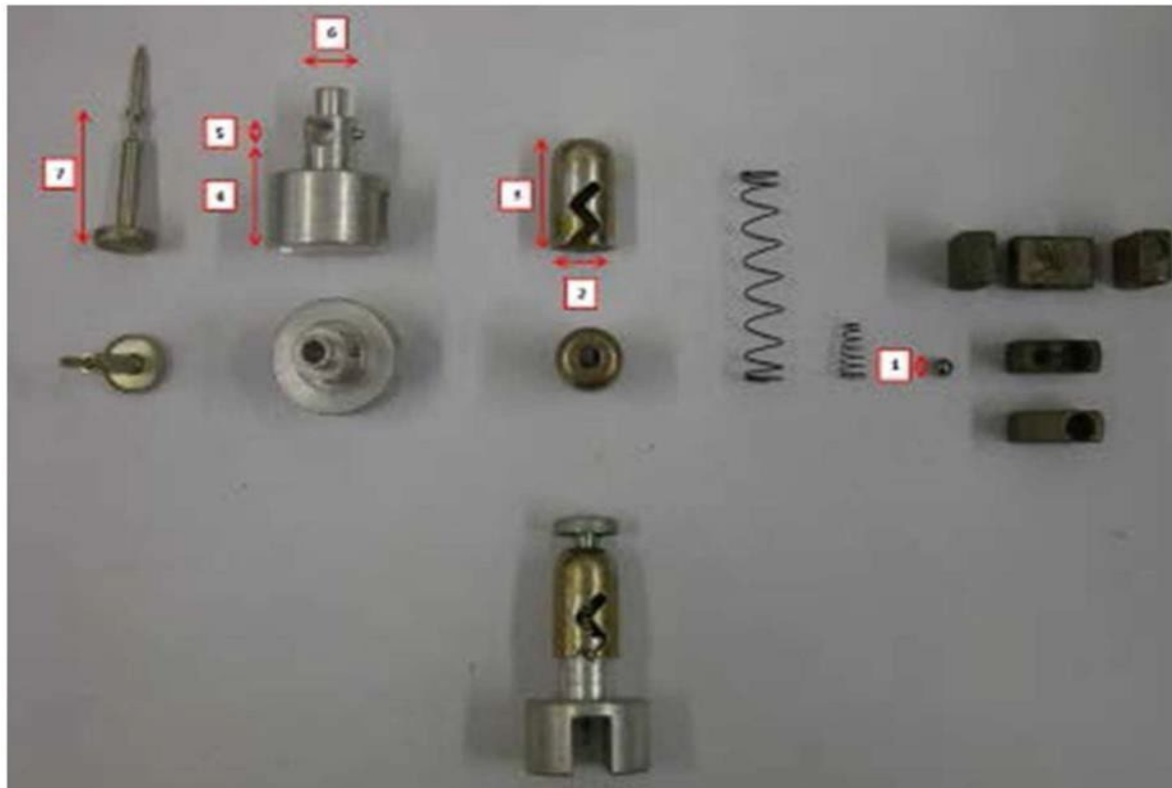
Figure 23: Fuse M6-N, Breakdown and dimensions measured by KC W&M. (Picture: KC W&M)
