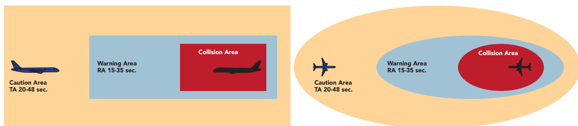
Figure 9: Schematic showing the vertical and horizontal plane, including the 'Traffic Advisory' and 'Resolution Advisory' regions 15
