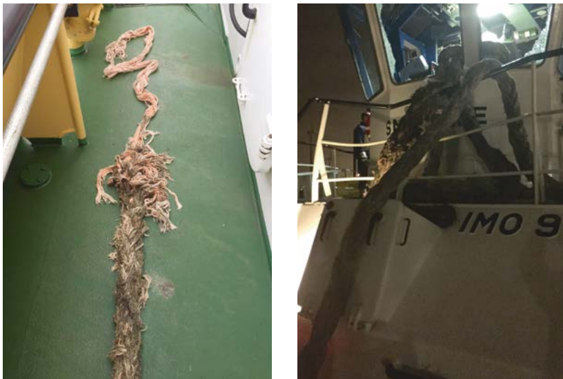
Snapped towage connection and damage to ship. (Photo: Boskalis)
