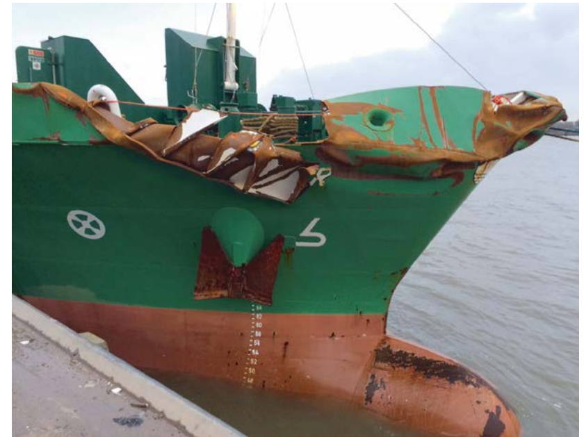
Damage to the freighter as a result of the collision. (Photo: Shipping company)
