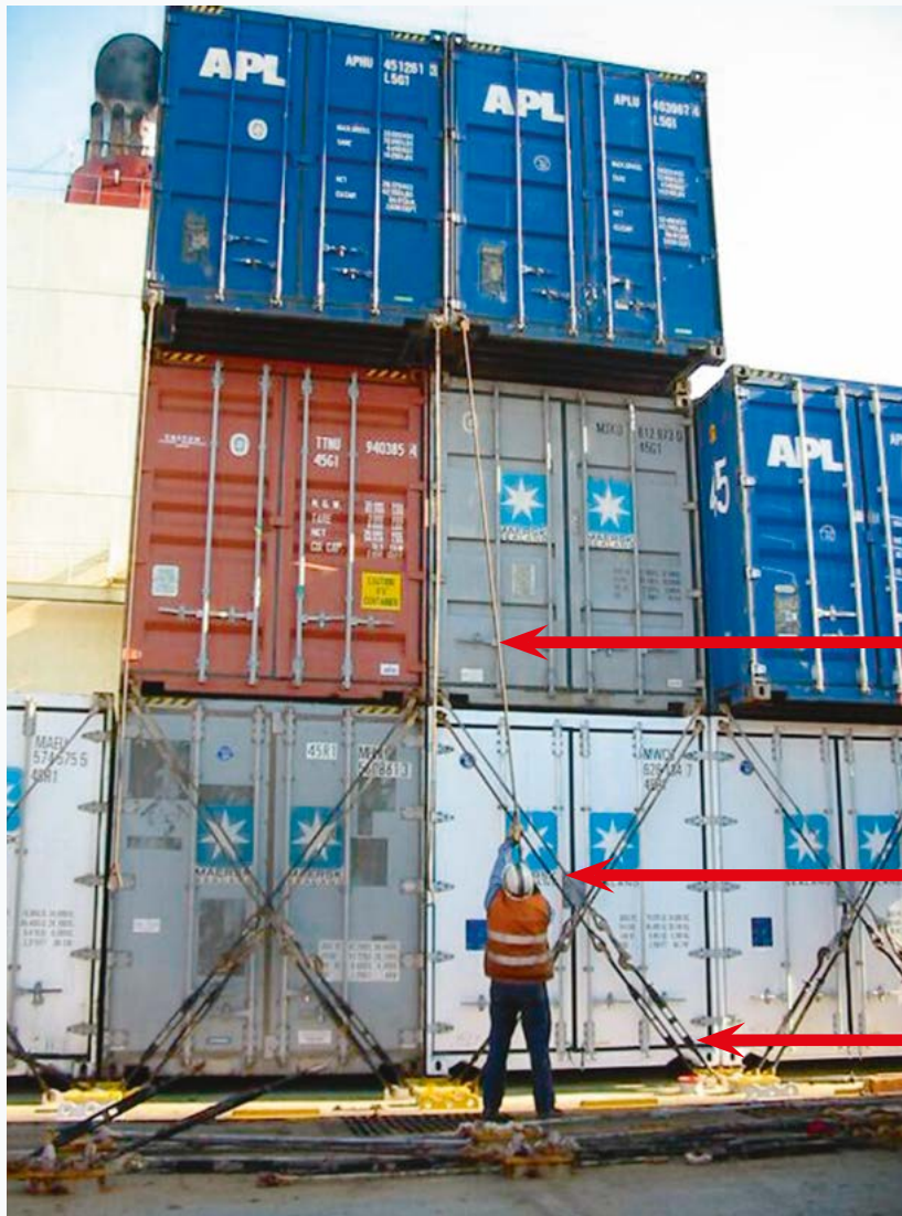
Stevedore secures a 5-metre-long lashing rod. (Photo: www.portpictures.nl – Danny Cornelissen)
