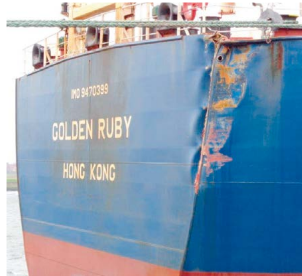
Dent in the stern of the Golden Ruby. (Photo: Human Environment and Transport Inspectorate (ILT))
