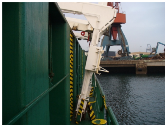
Photo 5: Position of the hatch crane on the starboard side in the gangway.
