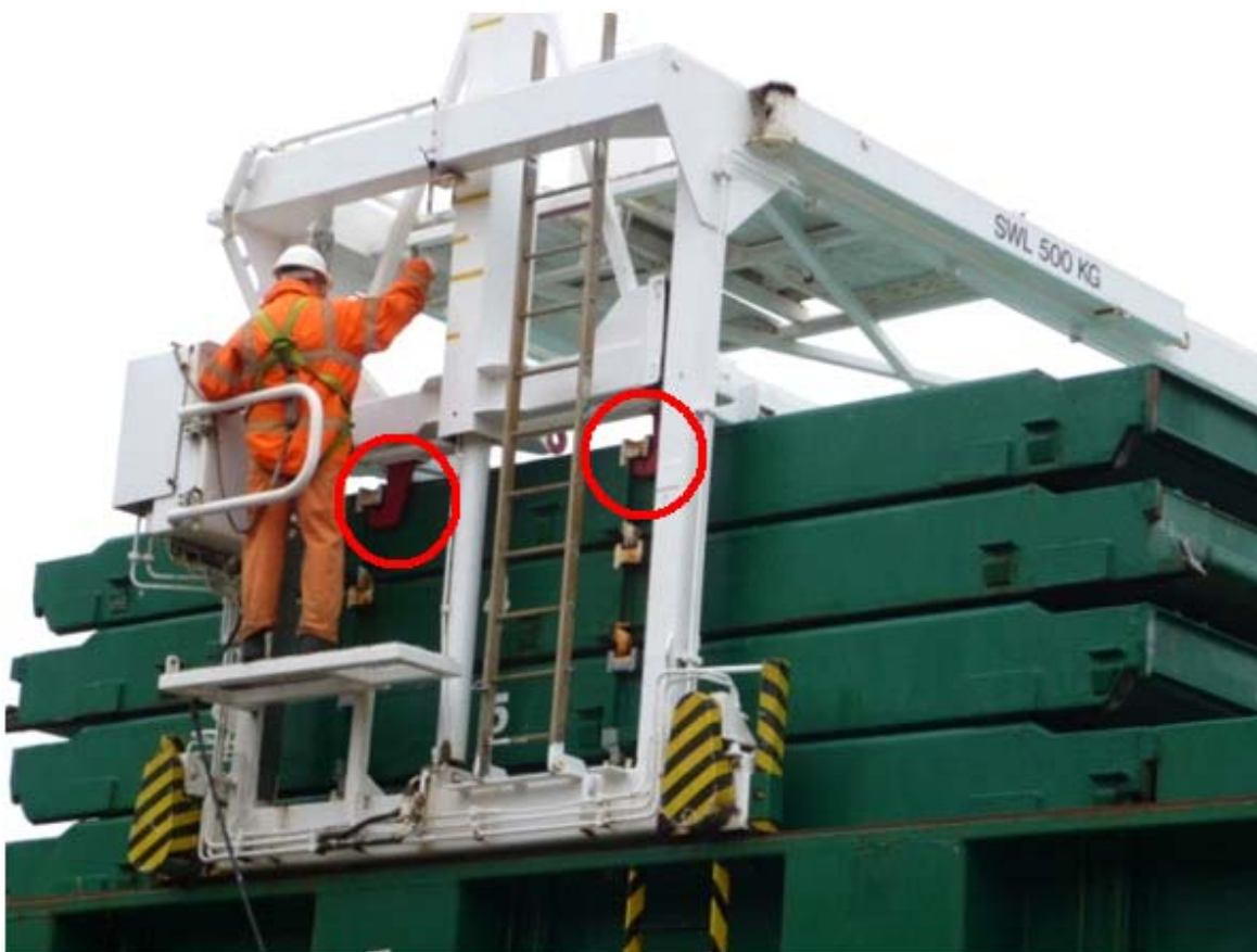
Photo 3: The hatch crane with hooked hatch (photo taken on the Arklow Sky in Sluiskil).
