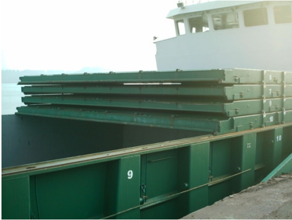
Photo 1: The piled hatch pontoons at the back of the hold, after hatch no. 6 had been driven away by the first mate.
