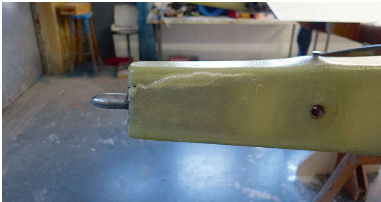
The tear in the left wing spar of PH-1006. (Photo: Flying club)
