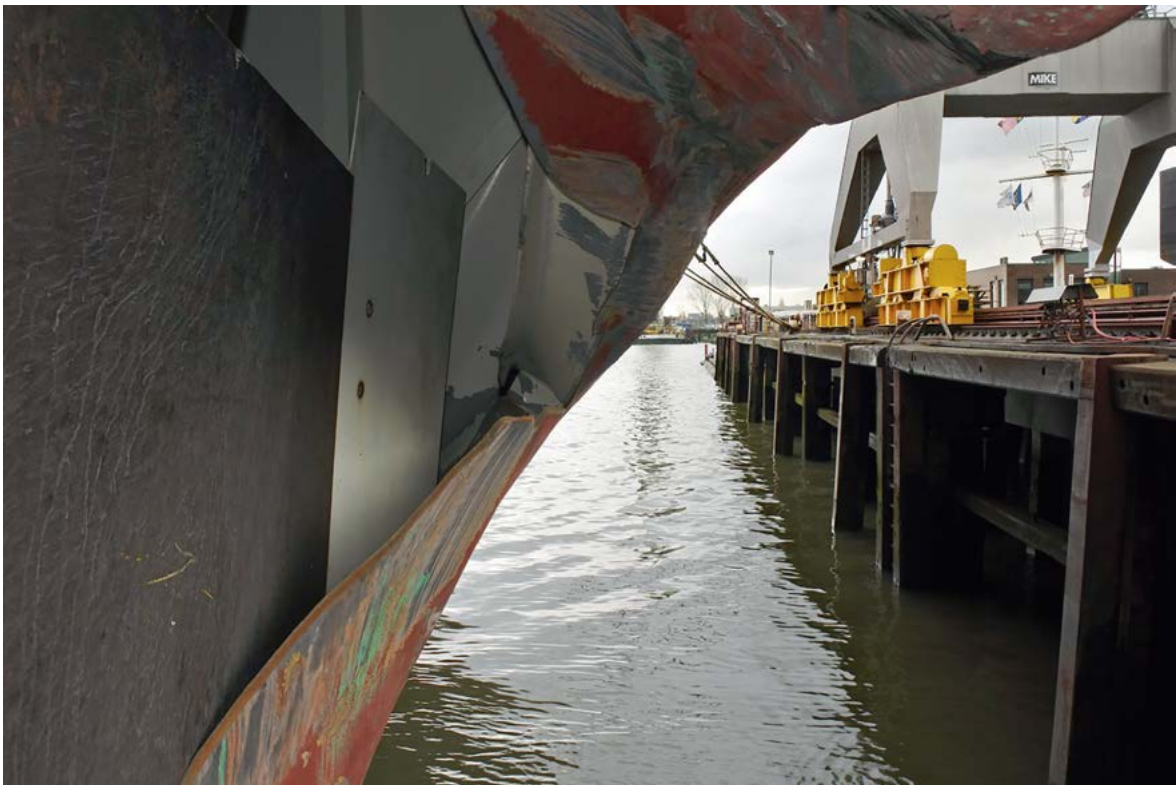
Figure 5: From inside the Atlantic Jupiter, looking out through the 15-metre long gash. (Source: Dutch Safety Board)
