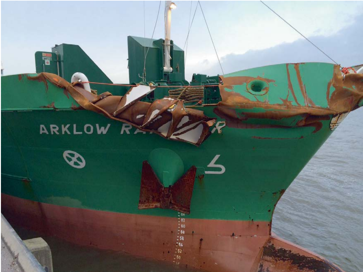
Figure 4: Damage to the bow of the Arklow Rambler. (Source: Dutch Safety Board)
