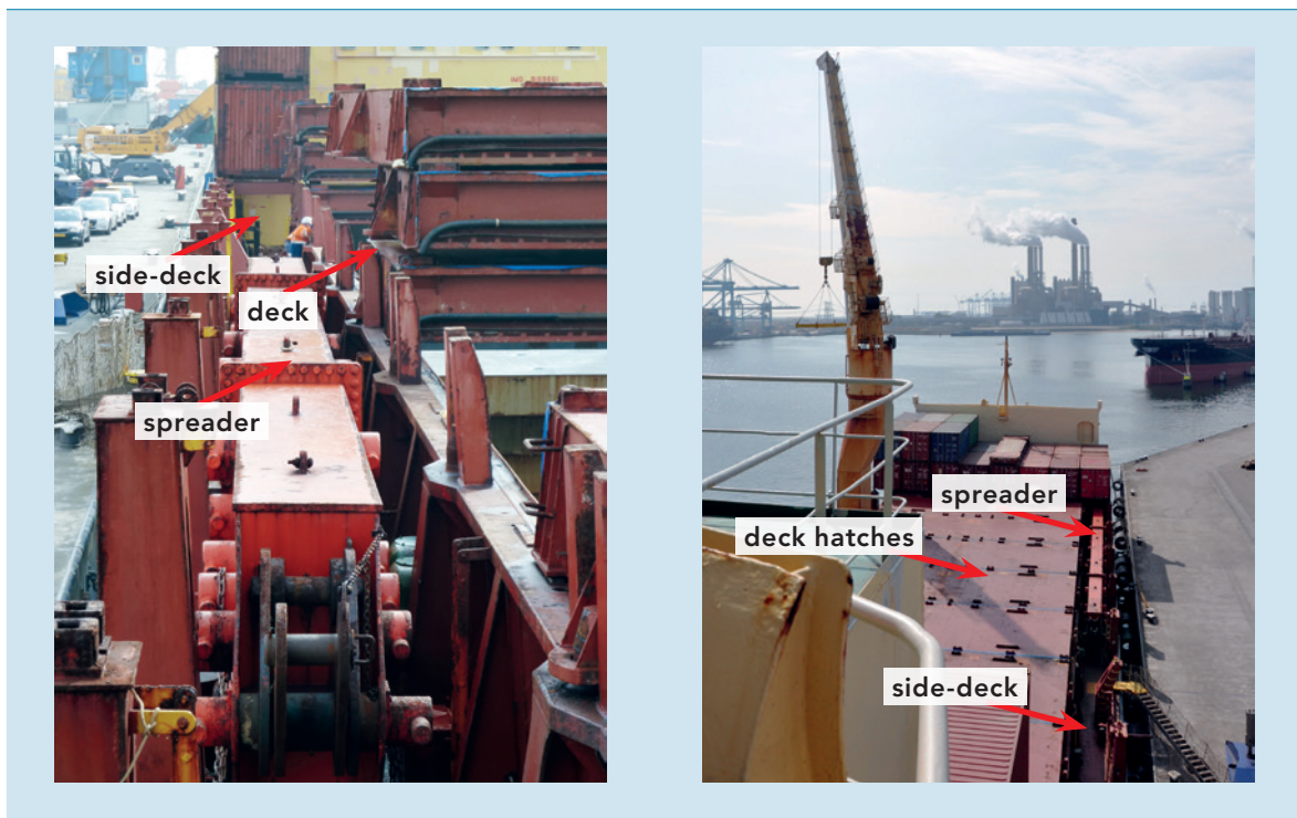
Figures 1 & 2: Hatches, spreader and side-deck. (Figure 1: Source IL&T, figure 2: Source: Dutch Safety Board)
