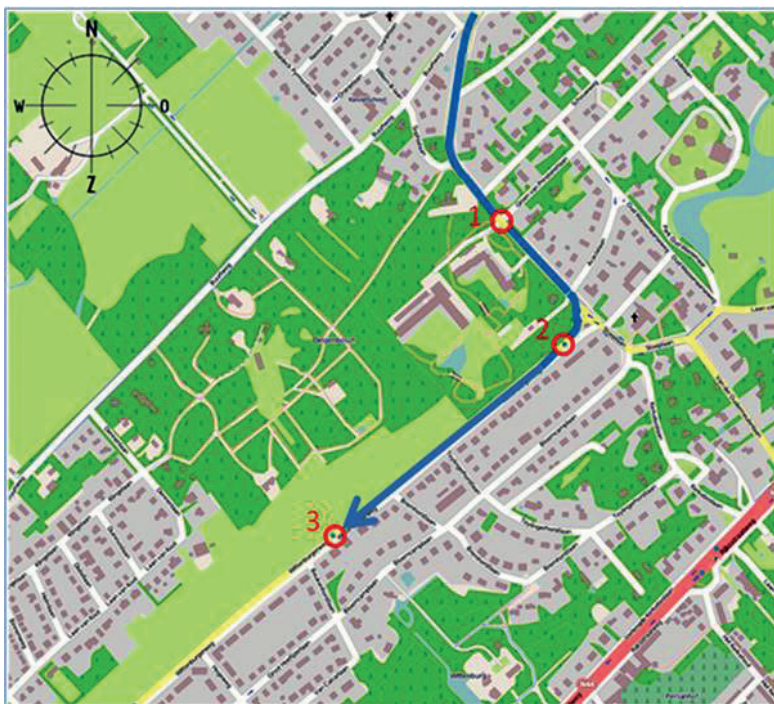
Figure 2: Route used by CNG-powered bus (blue line) in Wassenaar. Position 1: driver notices a burning smell. Position 2: grey smoke visible in rear view mirror. Position 3: driver stops bus at Beukenhorstlaan stop (Wittenburgerweg).
