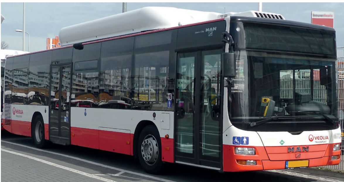
Figure 1: CNG-powered MAN Lion's City bus (with CNG system on the roof)
