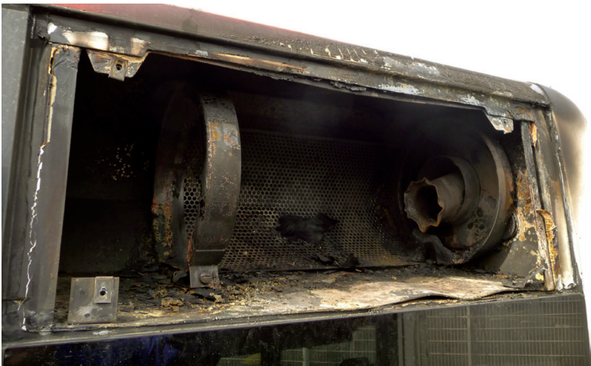
Figure 2: Fire damage to the engine air intake (after removal of safety grille)
