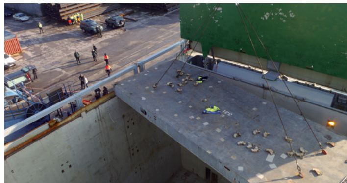
The pontoon shortly after the accident and simulated position on the stevedore platform without installed fall protection.
