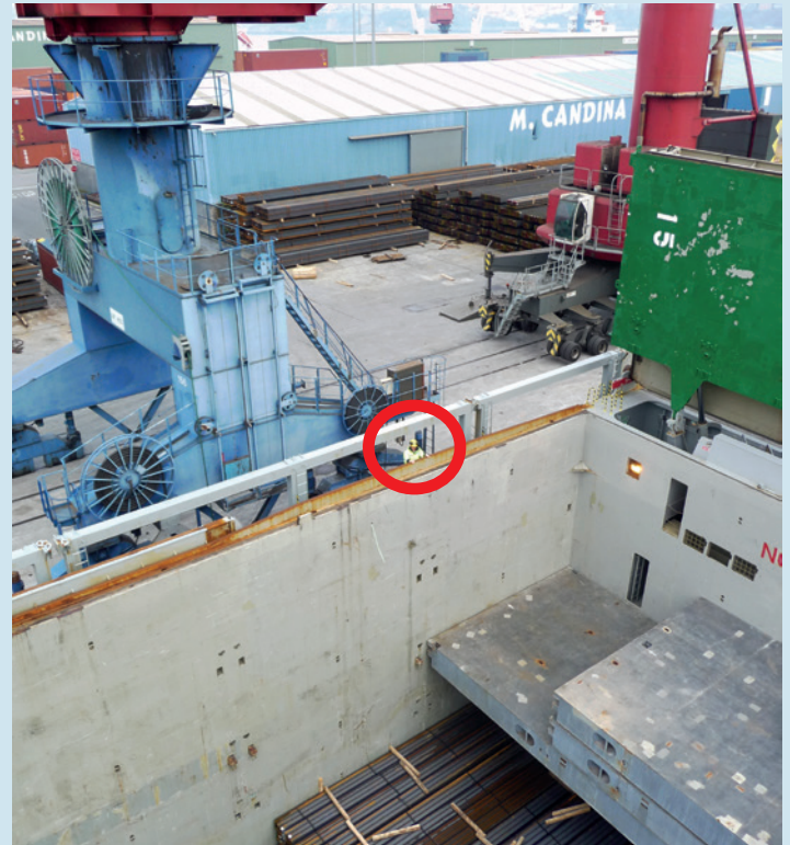
Simulated position of the chief officer from the crane driver's position.
