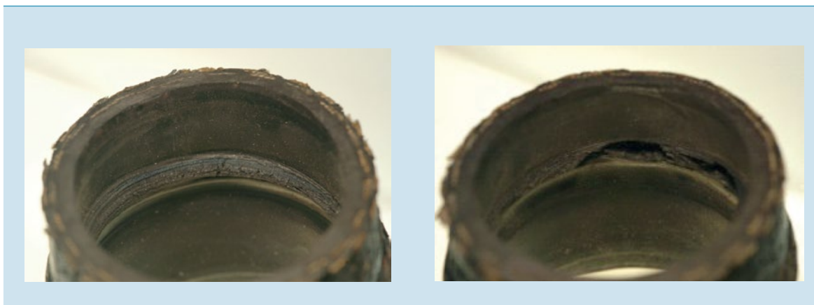
Figure 8: Hose with ridge, partly undamaged (left) and damaged (right). (Source: Dutch Safety Board)
