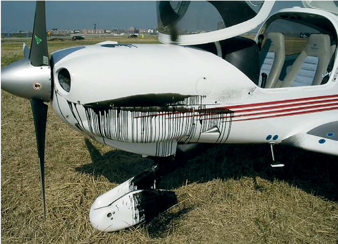
Figure 2: Engine cowling covered with engine oil. (Source: Wings over Holland)
