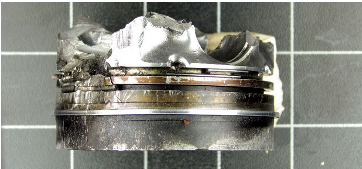
Figure 6: Piston number 3 with fire protection sleeve particle. (Source: BFU)
