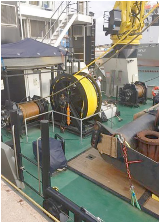
The drum with the umbilical cable (yellow) on board the Terra Plana. (Photo: BosKalis)
