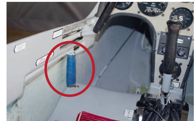
Airbrakes in unlocked position. (Photographs: captain PH-1252)
