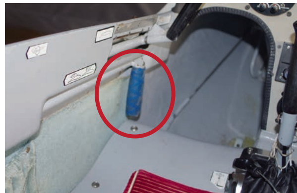
Airbrakes in locked position.
