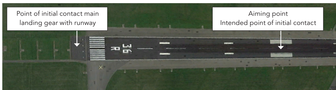
Figure 2: Top view of the first part of runway 36R with the initial point of contact of the main landing gear with the runway and the intended point of initial contact. (Source: Google Earth)
