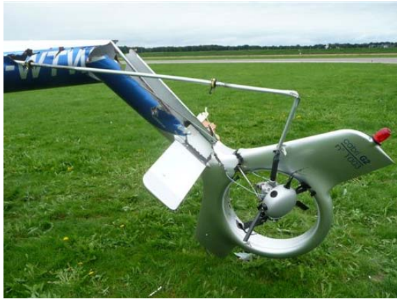
Figure 3: damaged tail and -tail rotor driveshaft Figure 4: flexible coupling
