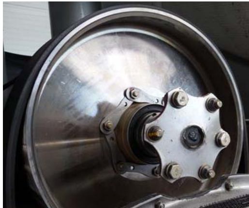
Figure 5: coupling stuck in airframe cowling Figure 6: engine driven pulley with bent coupling
