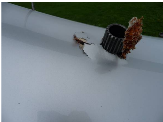
Figure 5: coupling stuck in airframe cowling Figure 6: engine driven pulley with bent coupling
