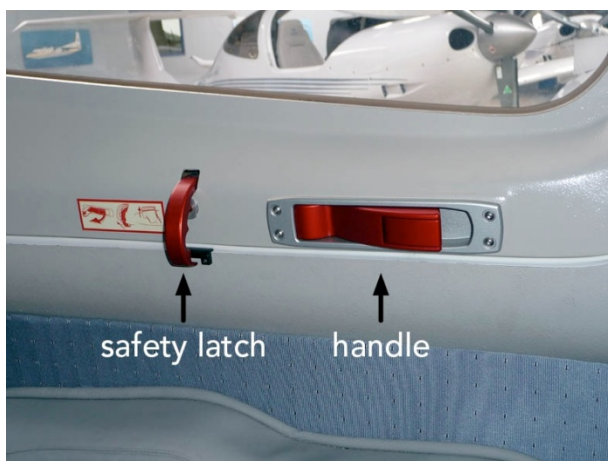
Figure 1: safety latch and door handle on the inside of the rear door
