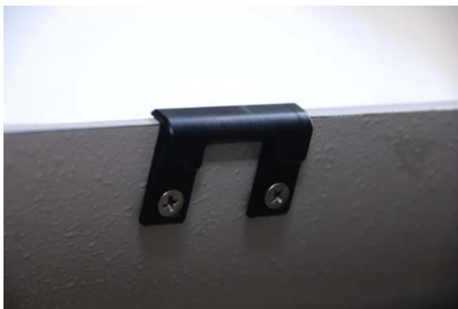
Figure 10: improved rear door retaining bracket of PH-TIN (source: W.L. Nijdam)
