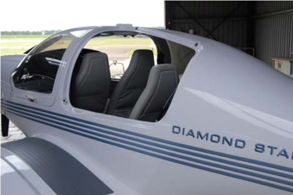
Figure 2: rear door missing after flight (source: W.L. Nijdam)
