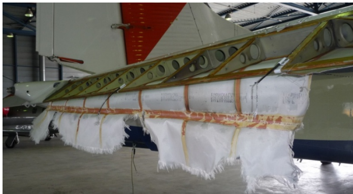
Figure 2: right hand elevator after the flight
