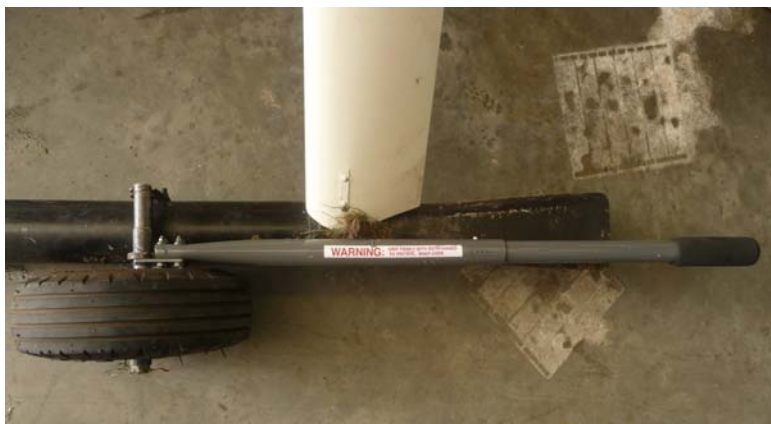
Figure 1: ground handling wheel with lifting handle mounted on left skid
