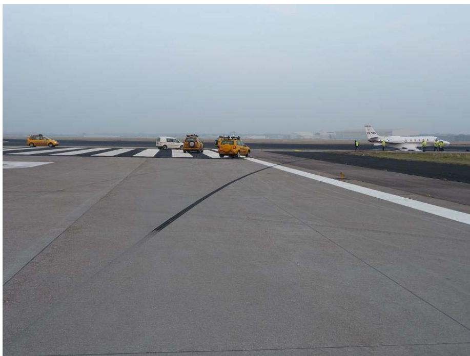
Figure 4: The CS-DXR after the event with the skid mark of the right main landing gear in the foreground.
