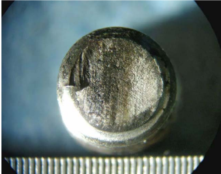
Figure 9: Enlarged fractured surface of the screw found in the lug of the left wheel [Source: Cessna].
