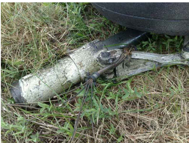
Figure 2: the failed left main landing gear outer tube
