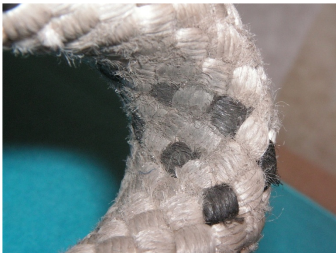
Figure 3: wear in loop at other end of launch restraint
