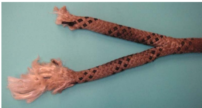
Figure 2: failed loop of the launch restraint
