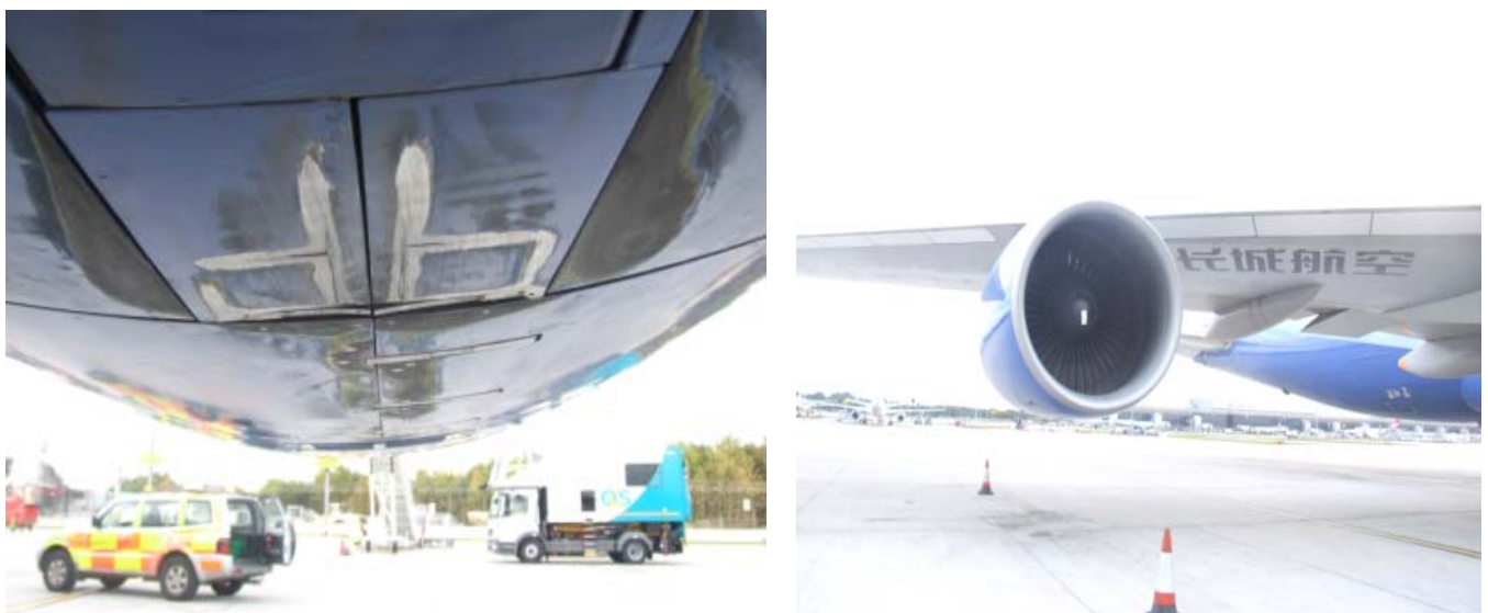
Figure 1: damage to the bottom of engine 4
