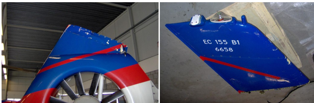
Figure 1: The lower part of the tailfin (left) and the separated upper part of the tailfin (right).
