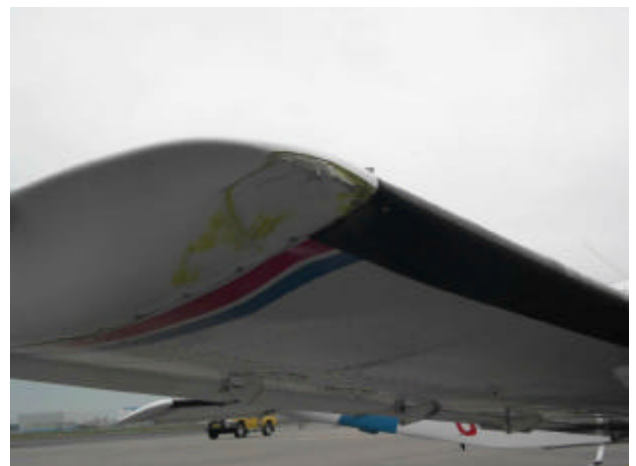
Damage to the right-hand wingtip
