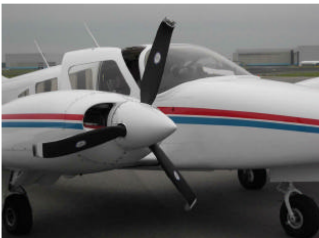
Damage to the right-hand engine propeller blades
