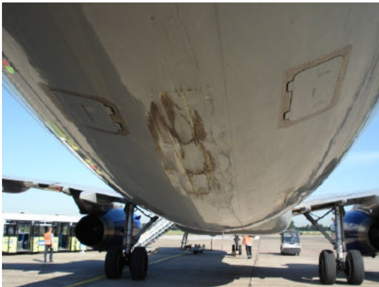
Figure 2: view on the aircraft's empennage with scrape marks
