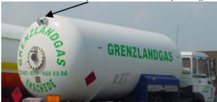
Illustration 10: Pressure relief valve fitted to the rear of a tank lorry (top)
