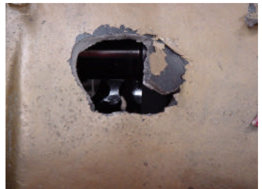
Hole in engine casing
