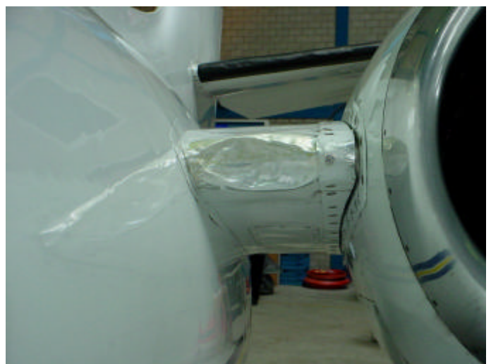
Dents in the aluminium sheet metal lining
