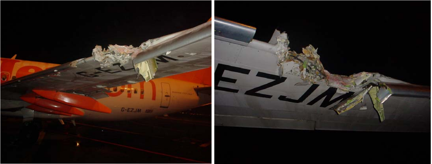
Figure 3: Photos of the damage to the left wing
