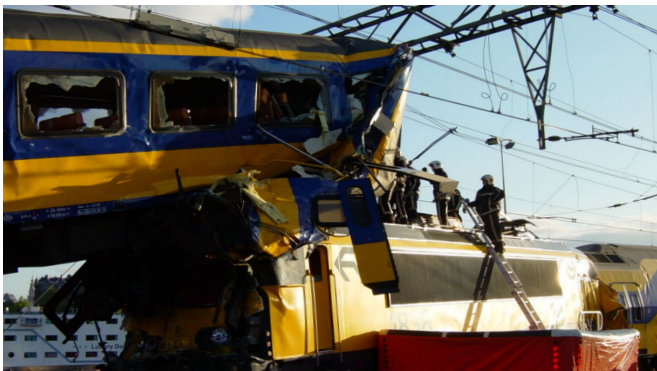
Figure B17. Amsterdam 21 May 2004. Train 80761 (empty double decker train VRM), following departure, passed stop signal 278. The double decker (right on the photograph) collided head on with the incoming intercity 960 from Utrecht. The first carriage of this passenger train was lifted up and folded double on the roof of the locomotive.
