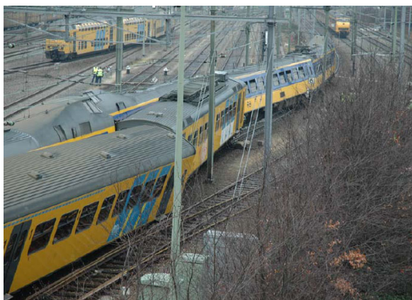
Figure B21. Rotterdam 11 February 2005. On the right the front section of stopping train 9725 (sprinter), which passed stop signal 254 and collided with the right flank of intercity 21723 (ICM).
