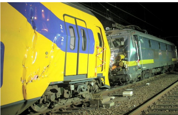
Figure B18: Diagrammatic track situation. On 30 September 2004, a double decker train, following departure, passed signal 216. For this train, a route had been set from track 4a to track 84. The train had to transfer to track VA. For a Belgian locomotive, a route was set from track EA to track 31. The two trains collided head on with one another. Assessment: This is a subroute which should have been avoided.
