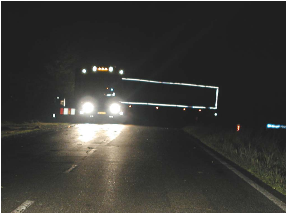
Illustration 8: photograph of the test situation with contour marking. (Source: TNO-TM)
