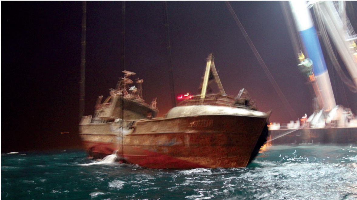
Figure 2: Damage to the starboard side of the Maria's seen during the first salvage attempt. (Source: Berex B.V., Zevenbergen)
