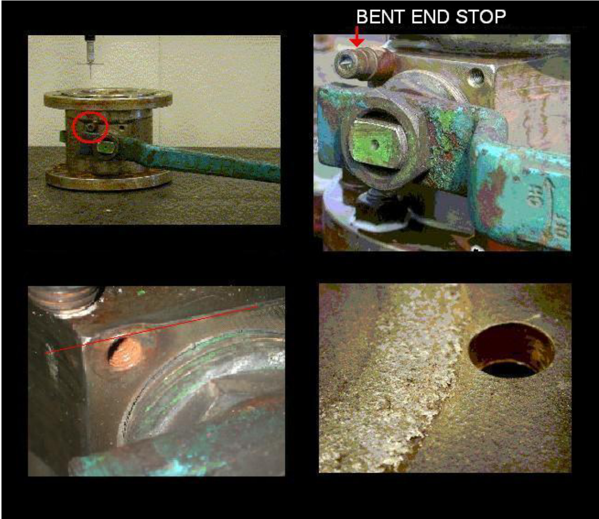
Fig.7. Top left. The stripped down stainless steel ball cock in a test bed. The handle has been pressed down until it comes into contact with the bent end stop. Even then, the cock is not closed. The handle is then not horizontal. In its horizontal position (closed position), the cock is parallel to the side of the table on which the ball cock is mounted. This ball cock has the special feature that there are only two positions in which the cock is closed. In all other positions, the cock is opened.
