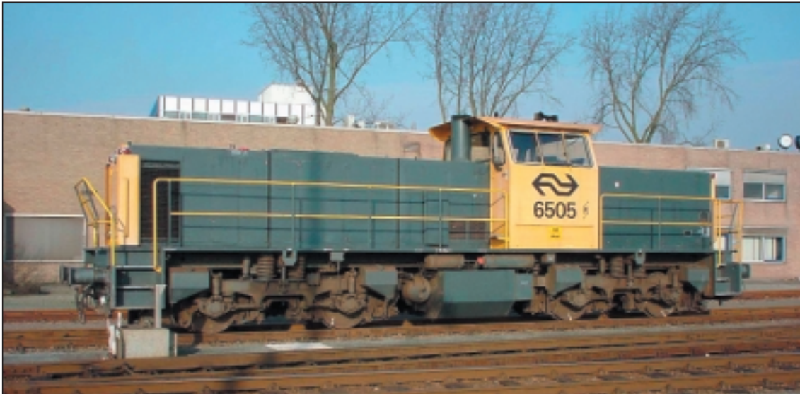
Fig. 7 The locomotive remotely controlled by radio signals, operated by Railion. In the background the office building, containing the traffic control post.
