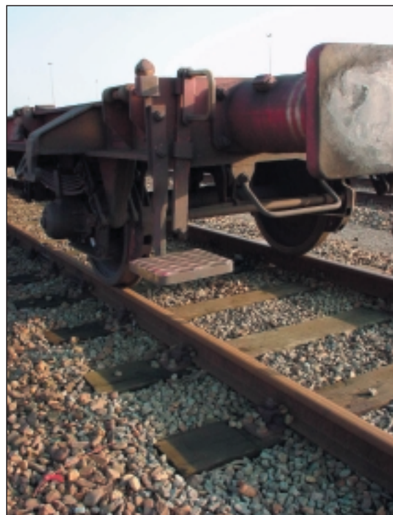
Fig. 8 The internationally-standardised footboard on freight wagons. The handle is first raised, and then acts as a support.
