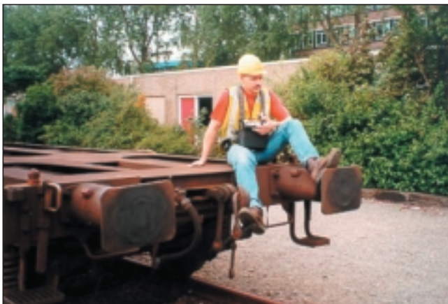
Fig. 4 Position of radio-controlled train driver. The control box is held in front.
