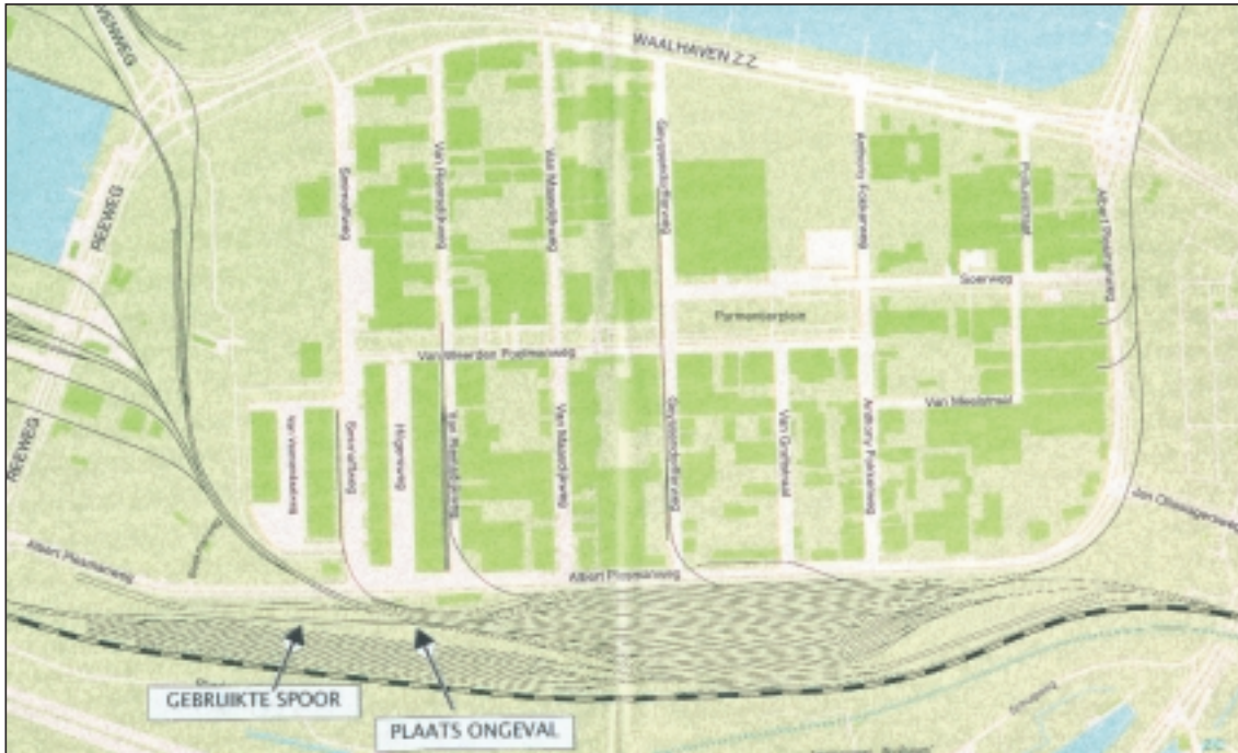
Fig. 2. Waalhaven marshalling yard with connection tracks to companies. On dead-end tracks, push-shunting is unavoidable.
