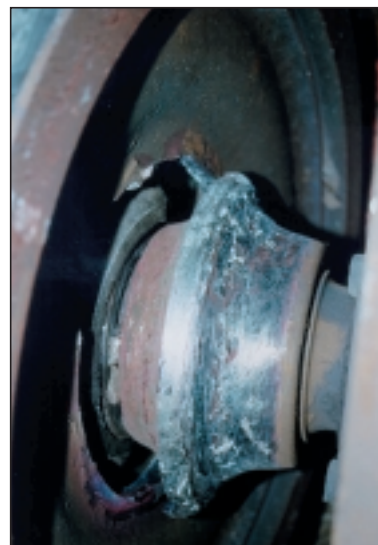
Fig. 7 The cracked inner wheel
