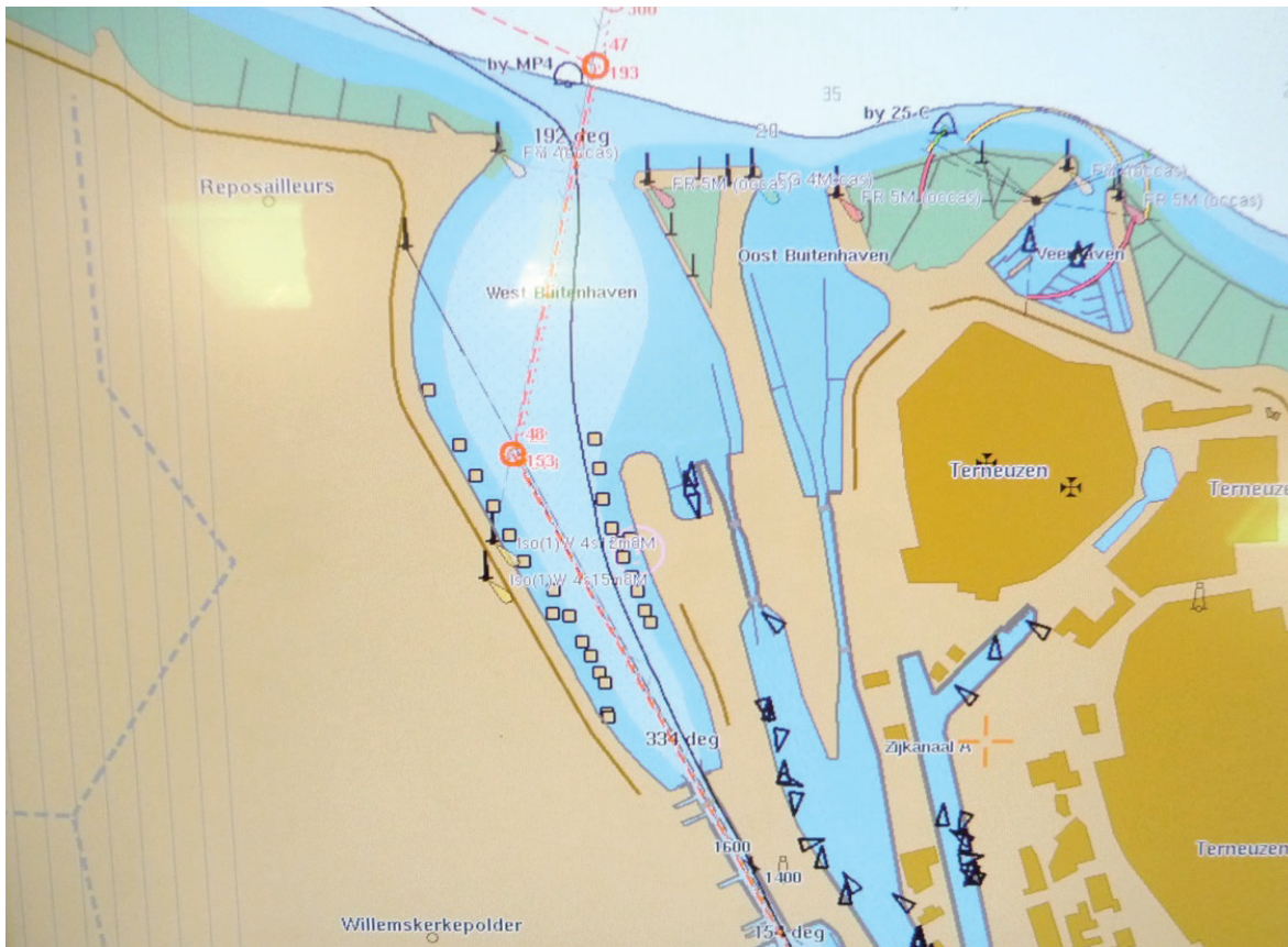
Figure 2: Image of the track (in black) of the Flinter Aland on the display of the electronic chart system (ECS).
