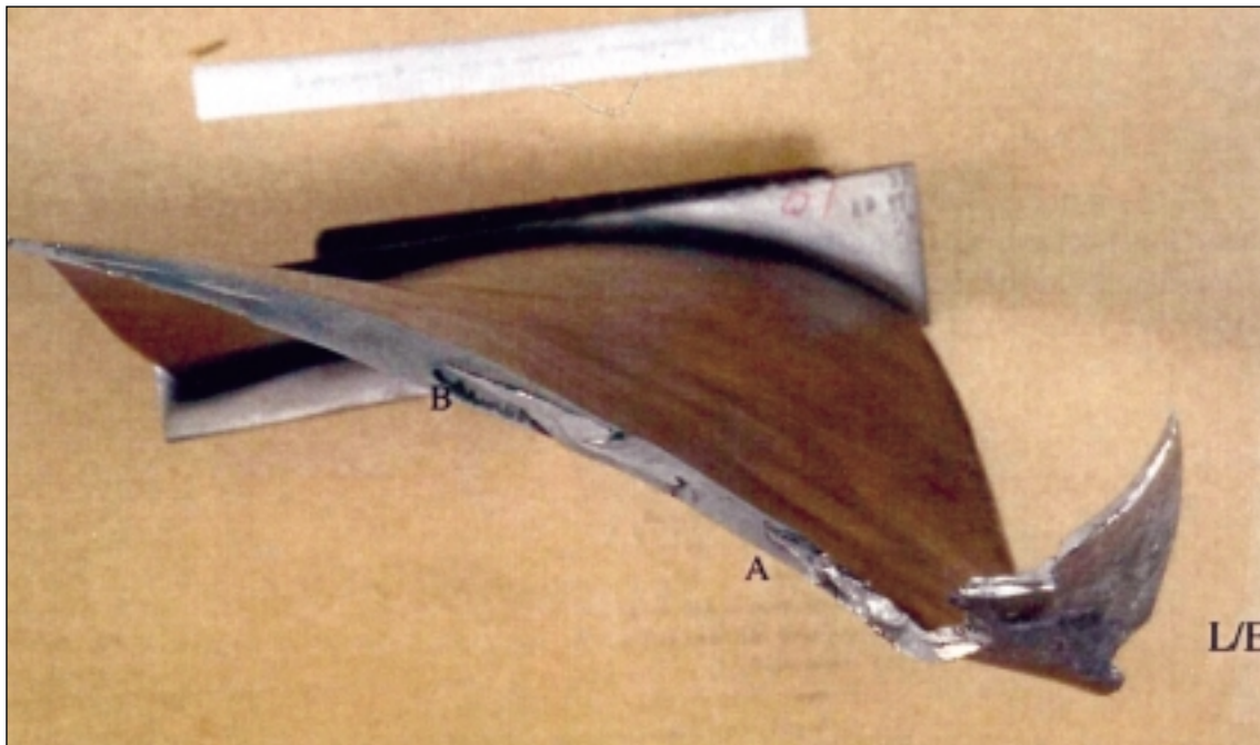
Figure 5: Inner airfoil fracture surface of fan blade 10
