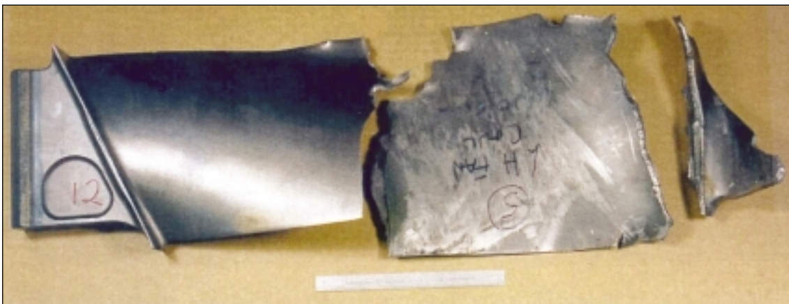
Figure 1: Inner airfoil and recovered parts of fan blade 12
