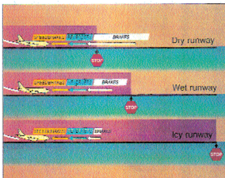
Figure 8. Stopping forces. The total stopping force available is the sum of the drag, reverse thrust and braking components. The total force determines the deceleration and thus the stopping distance.
