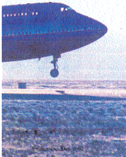
Figure 1b. Dynamic hydroplaning. At high speed the tire planes on deep, standing water. Tire grooves and runway surface macrotexture (slippery or grooved surface) help drain water from the footprint and improve friction.
