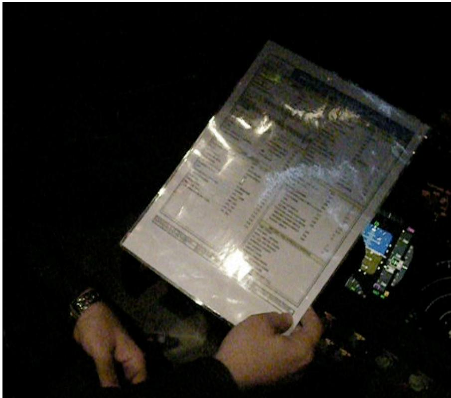
*A THY landing checklist being accomplished in a B737NG cockpit (left seat). The checklist, held between the left-seat pilot and the control yoke blocks the view of the PFD (Primary Flight Display) which includes the airspeed tape (Photograph: Author).*
