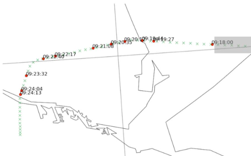
The aircraft is flying on a westerly heading. The crew is slowing the aircraft down from over 300 KIAS to 250 KIAS during this time, while descending from FL080 through FL055. At 09:15:58, amidst a flood of clearances to other aircraft on the approach frequency, TK1951 gets a clearance from the approach controller to fly to SPY (Spijkerboor VOR) and expect the ILS for runway 18R. It is around 35 track miles away from the touch-down point on runway 18R.
